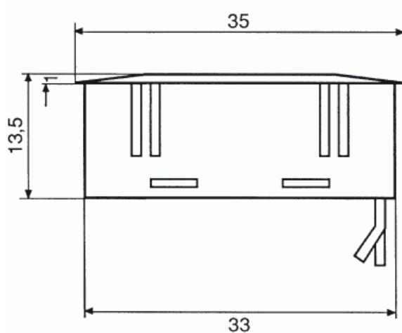
The light indicator is fitted in the hole from the front of the panel.
