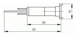
The lens is inserted from the front of the panel. it fits in the case of the light indicator situated behind the hole in the back of the panel.
