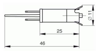
The lens is inserted from the front of the panel. it fits in the case of the light indicator situated behind the hole in the back of the panel.
