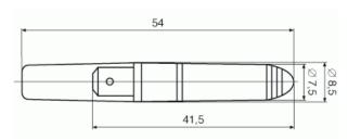
Light indicator with conical lens to be locked in the panel hole 10 - 12 - 13mm diameter. It can be assembled with the following types of lens: SRZ - SDY - SDK - SFY.
