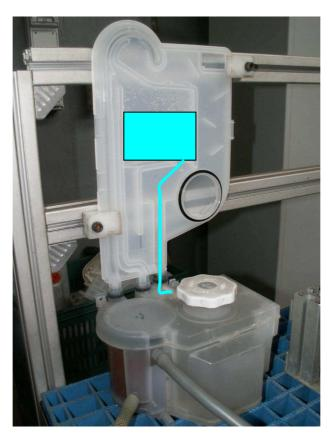
Regeneration valve is energized, so to release the potential energy of the water amount above, in the air-breaker, and allow a movement of water:
